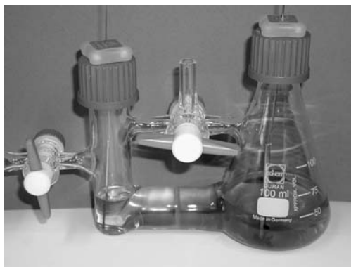
Fig. 3.10. Schematic sketch and photograph of an electrocrystallization cell. As a different design, H-type cells are often used. Single crystals of \kappa\text{-(ET)}_2\text{Cu(NCS)}_2 are formed at the anode (right electrode). Note the change in color of the solution between the cathode (left) and anode side (right) after growth time of several weeks. The glass frit serves as a filter which prevents the chemical reaction products on the cathode side from diffusing to the anode side.
